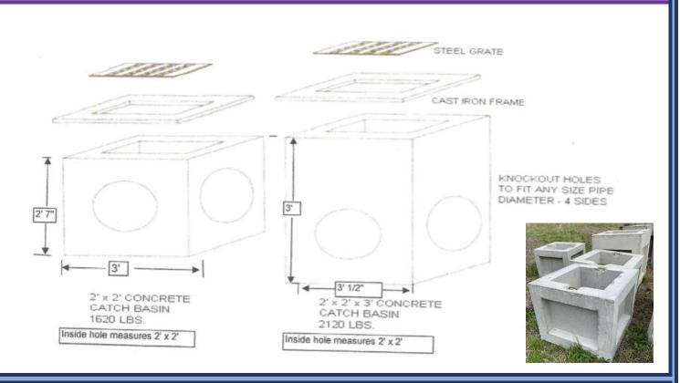
USED FOR STORM DRAINAGE APPLICATIONS, 2' x 2' OUTSIDE DIAMETER, 6" CONCRETE WALLS, 3500 PSI CONCRETE WITH REINFORCED BARS
